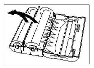
(3) Remove the old film roll from the cartridge.
